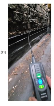
No trace of gas from termination or brickwork under decking.
