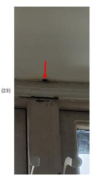
Test rig 2b pipe inserted in hole at centre, again positive readings on exterior brickwork.
