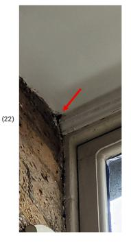
Test rig 2a involved inserting gas pipe in small hole in corner, positive reading on exterior brickwork.
